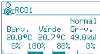
The display example on the left shows regulation in three steps, where the first step is a cooling step. The second step is a heating step with 100% output and the third step is a heating step with 80% output.
