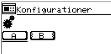
**The gear symbol** is displayed while the unit works to import or save a configuration.
